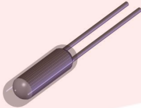
Fig. 3: Wire-wound glass resistor (M-GL)
