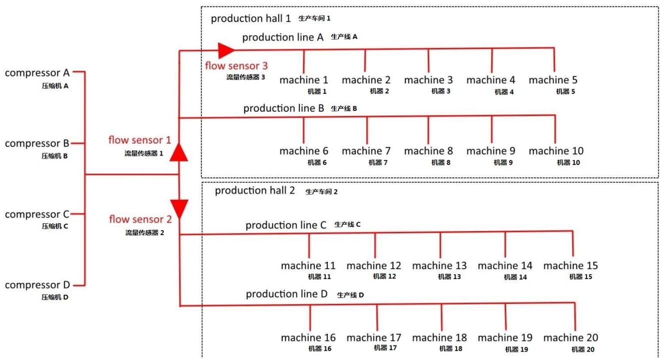
Now you know that production line A needs about 4000 Nm<sup>3</sup> of compressed air per day. That means that production line B only needs 1000 Nm<sup>3</sup> per day because line A and B together need 5000 Nm<sup>3</sup> per day.
