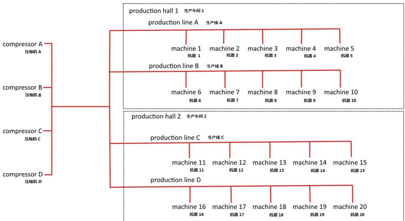
Where would you start to reduce leakages? If you don't know the compressed air consumption of your production halls, production lines and machines then you don't know where it is reasonable to start reducing leakages.
