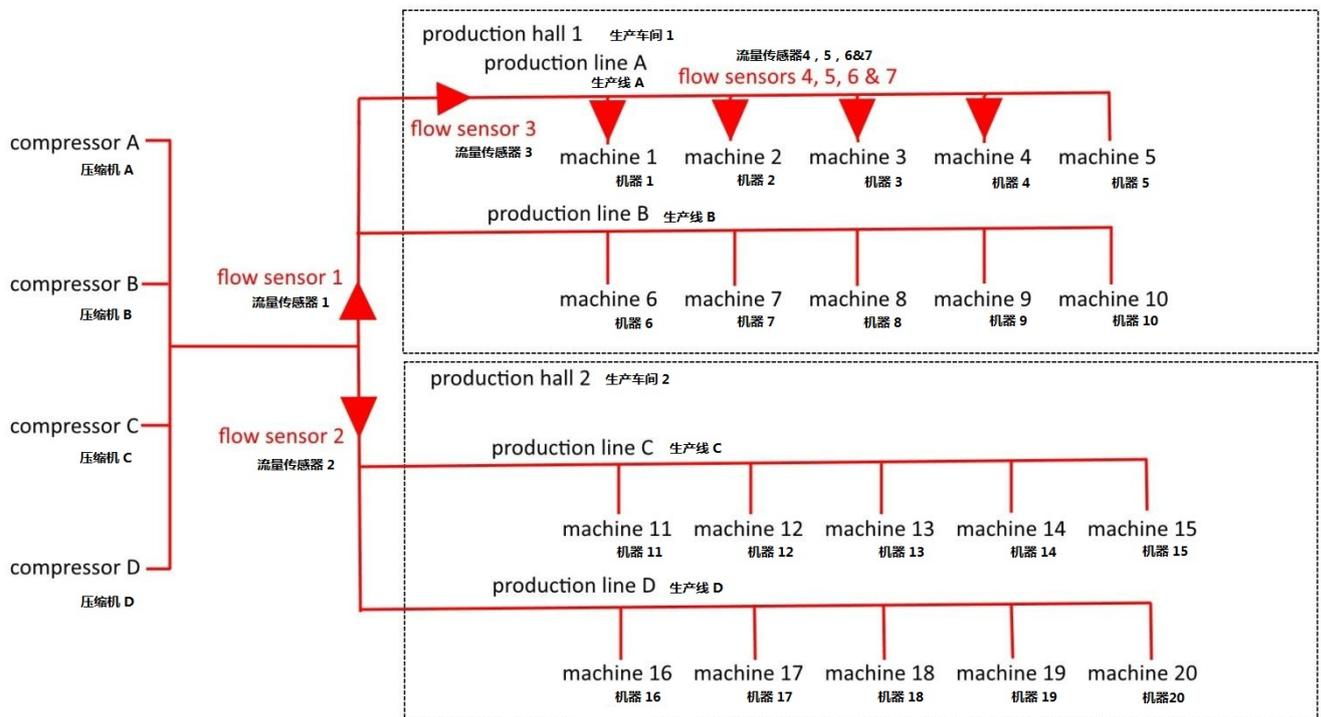
Now you know the compressed air consumption of every machine. So if you observe the compressed air consumption of your halls, lines and machines, you will notice if for example machine 2 needs much more compressed air as usual. So you can decide where it is most important to reduce leakages next.
