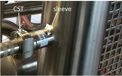
For installation of CSP the customer always additionally needs a sensor adapter TP or a ball valve BV. 对于安装CSP,客户总是需要一个传感器适配器TP或一个球阀BV。
